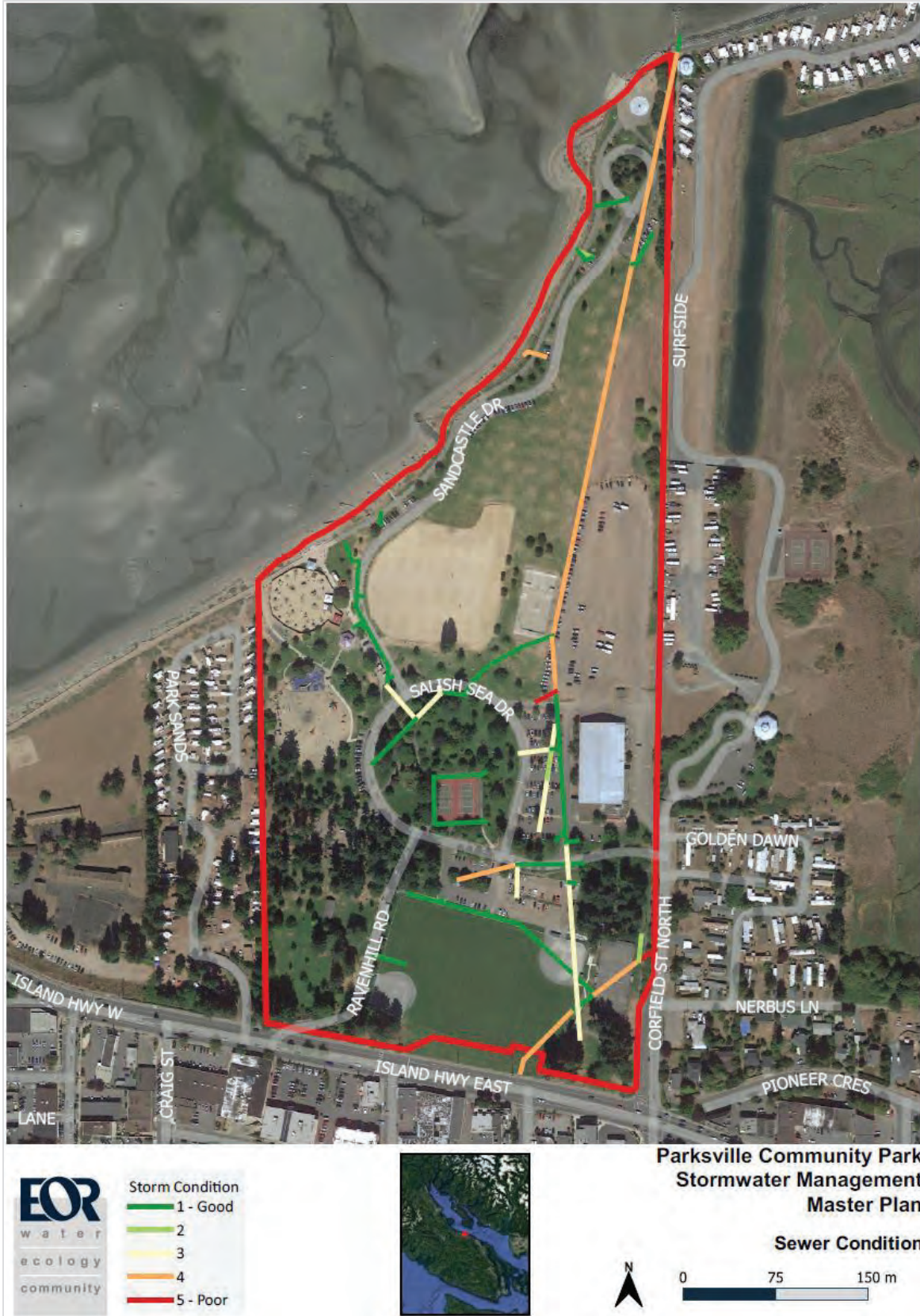
Figure 18. Estimated Sewer Condition
