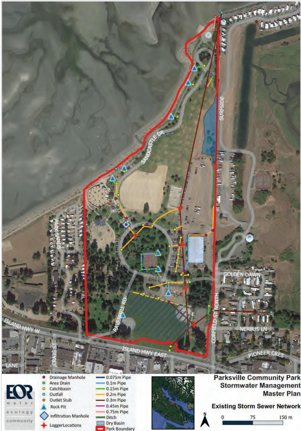
Figure 17. Existing Stormwater Management System
