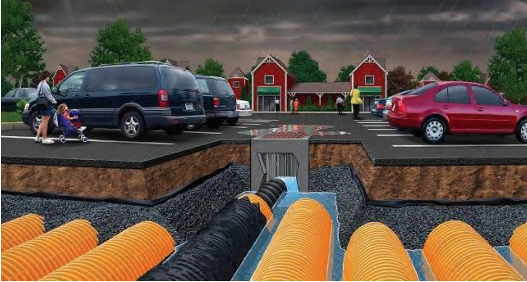
Figure 29. Example of underground storage facility for reuse
