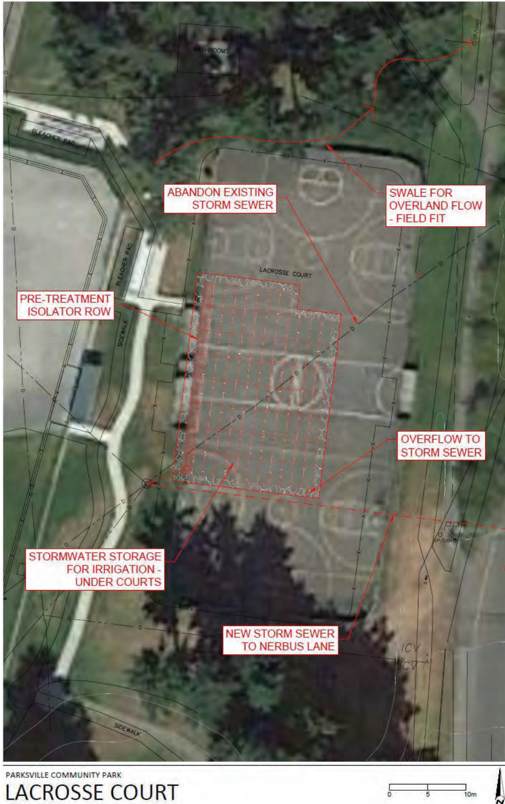
Figure 28. Concept design for stormwater infrastructure upgrades and regrading address deficiencies in the Southeast catchment with optional stormwater storage for irrigation
