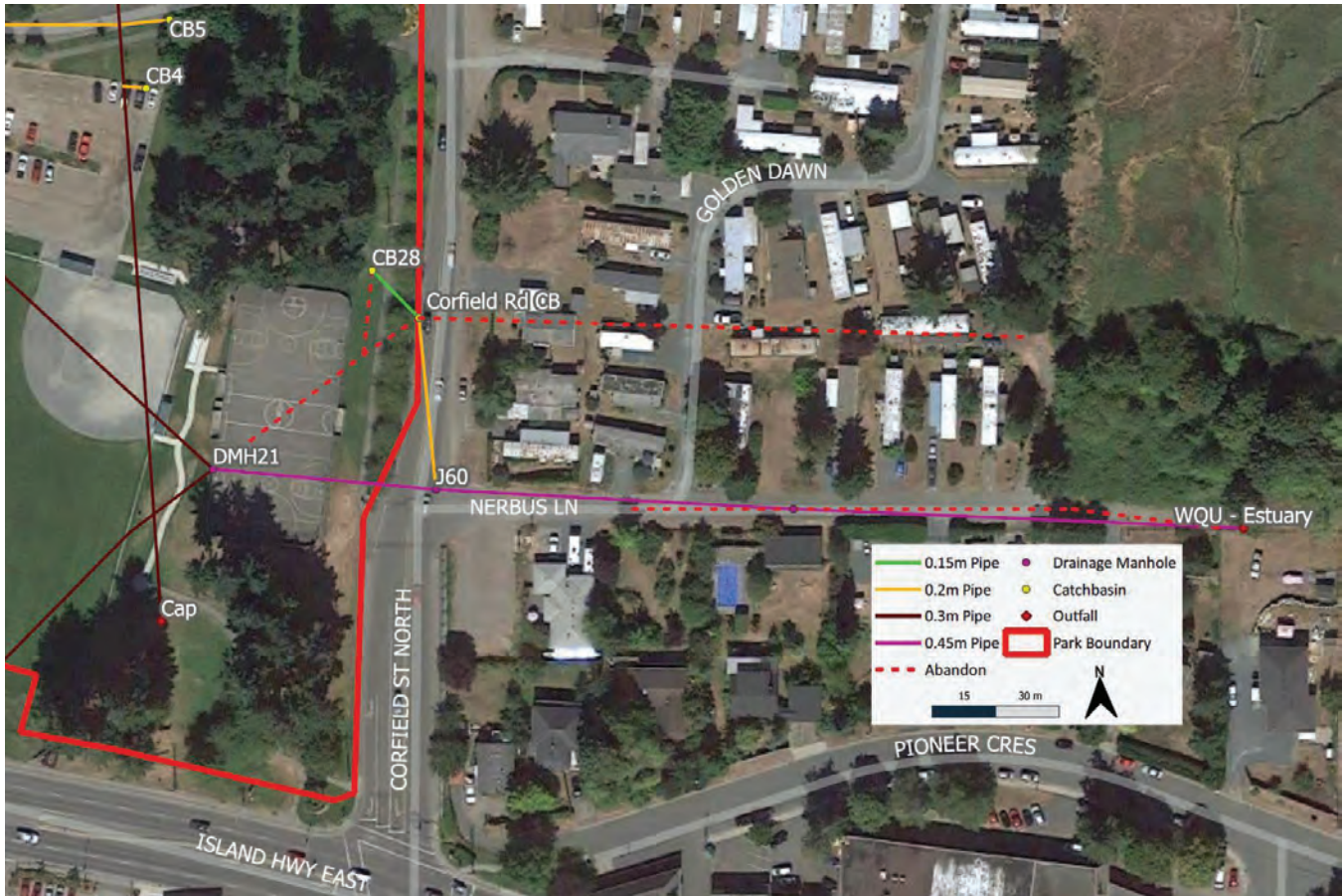
Figure 27. Nerbus Lane storm sewer connection concept
