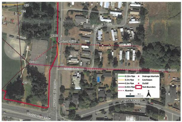
Figure 8. Nerbus Lane Realignment Concept Plan
