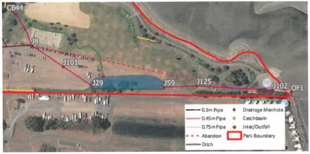
Figure 10. Dry Pond & Stub Connection Concept Plan
