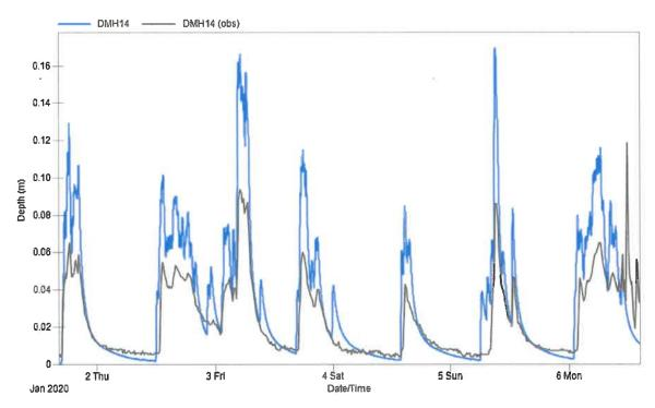
Figure 13. Waterlevel calibration at DMH 14. Displayed time period differs from other locations because of issues with monitoring data.
