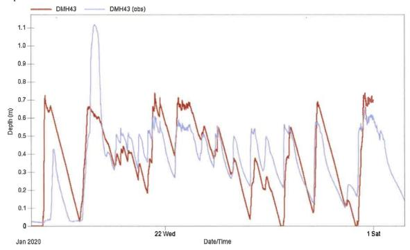
Figure 9. Waterlevel calibration at DMH43. Time period differs from other locations because the system response is significantly different.
