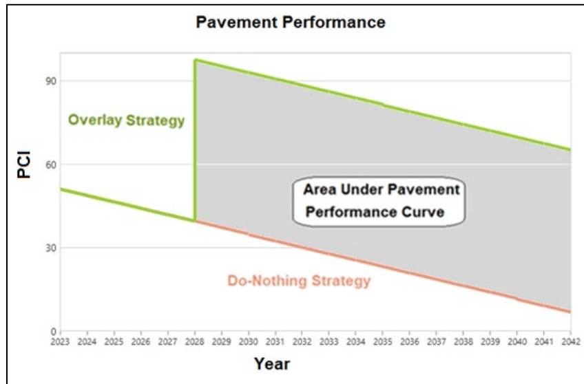
Figure 14: Example of calculating the benefit for an Overlay Strategy
